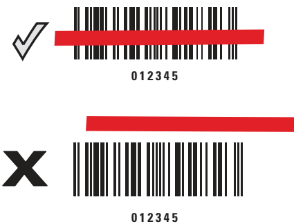
Figure 2-6 Scanning Orientation with Aiming Line
